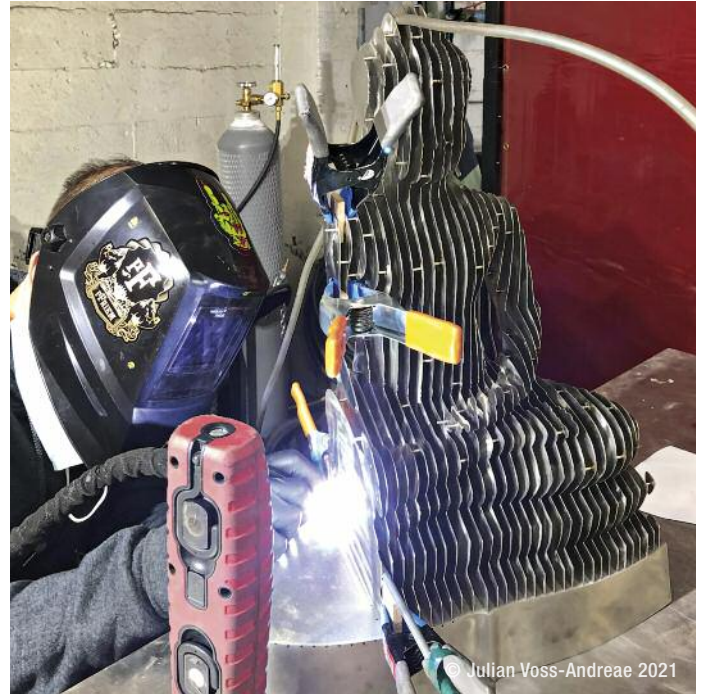
➤ Each panel is plug welded onto the dowels of the last, then it is resanded and polished.
